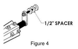
through. It is possible to remove any existing frame bolt and replace it with the supplied bolt in the bracket kit. **Recommended torque for the 5/8 x 2-1/2" bolt with washer is 110-115 ft-lbs**
