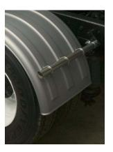
**NOTE:** Depending on the length of the truck frame and the placement of the mud flap hangers, the fender may tuck inside the mud flap hanger.
