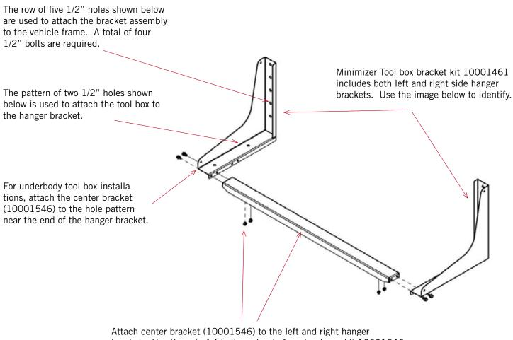
brackets. Use the set of 4 bolts and nuts from hardware kit 10001546 shown above.
