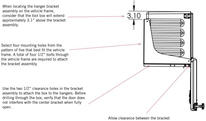
Allow clearance between the bracker assembly and the door when in the open position.
