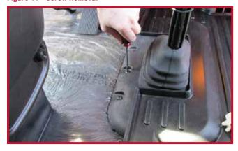
b) Insert the screw through the hole in the retention hook as shown in Figure 12.
