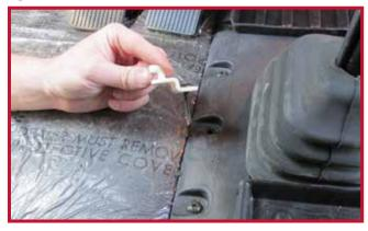
c) Insert the hook through the hole in the transmission cover and tighten using a #3 Phillips screwdriver. Orient the hook so it points straight toward the gearshift as shown in Figure 13.
