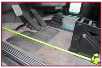
Measure from the lower kick panel of the dashboard to the front of the seat base. This measurement will determine the correct kit for your truck.
