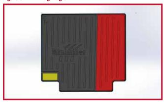
6. Trucks with a 18 speed transmission that are equipped with a MX13 Paccar engine require hand trimming of the passenger mat for proper fit around the gearshift. As shown in Figure 7, draw a line on the floor mat 1.75" away from the inside edge of the front lip around the gearshift. Use a utility knife to trim the floor mat material along the line. After trimming, the mat will lay properly in the truck as shown in Figure 8.
