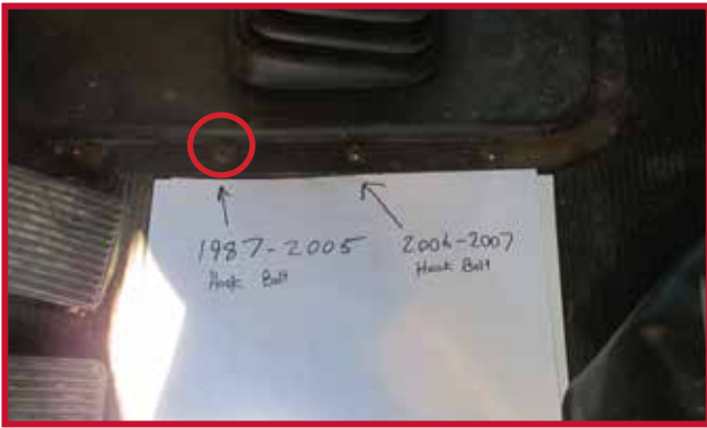
Figure 5 - Mounting Screw Identification
