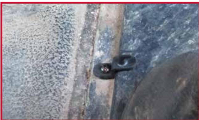
Figure 7 - Proper Hook Orientation
