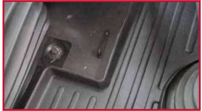
Figure 8 - Properly Installed Retention Hook
