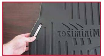
9. Once the hook is in place, let the driver mat and hook rest on the truck floor.
