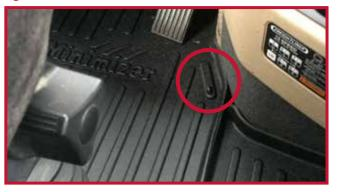
17. Pull the driver mat toward the rear of the truck to confirm that the hook is fully engaged into the mat and that the hook is adhered to the floor. If the hook is not functioning properly or the mat cannot be securely installed, do not use a Minimizer floor mat on the driver side of the vehicle.
