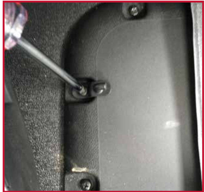
Figure 8 - Retention Hook Installation
