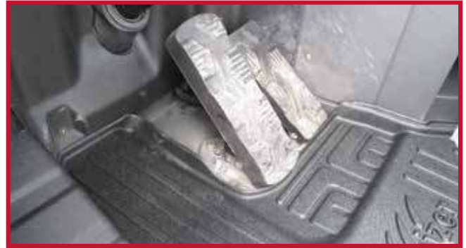
Figure 3 - Driver Mat Contact with Kick Panel
