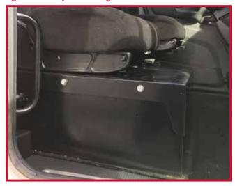
• Raised trim lines are available to fit the passenger seat with battery box seat base as shown in Figure 9.
