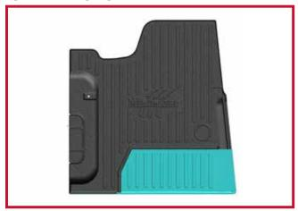
• Trim the teal shaded area of the floor mat along the raised rib to fit the battery box seat base.
