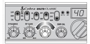
1 Rotate O Delta-Tune knob to the center position for optimum tuning.
