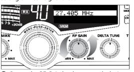
Rotate the RF Gain knob counterclockwise to reduce gain in strong signal areas. In weak signal areas turn clockwise to increase gain.
