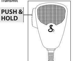
Push and hold mic button to transmit. Transmitter is now activated. When transmitting, hold the microphone two inches from your mouth and speak in a clear, normal voice. *Release* to receive.
