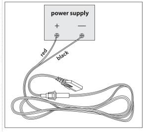
• Simply connect the red (+) and black (-) leads of the transceiver to the corresponding terminals of the power pack.
