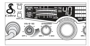
• Full *counterclockwise* rotation opens the "gate" allowing all signals in.
