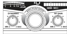
Select one of forty channels and adjust volume. The selected channel (1 through 40) will be indicated by the readout directly above the channel selector knob
