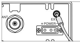
• Connect an external speaker to the external speaker jack on the rear panel.
