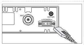
6 Plug the power cord into the jack marked "Power" on the back of the unit. Be sure to observe polarity markings.
