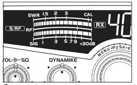
• The S/RF-SWR-CAL switch must be in the S/RF setting to read the meter.
