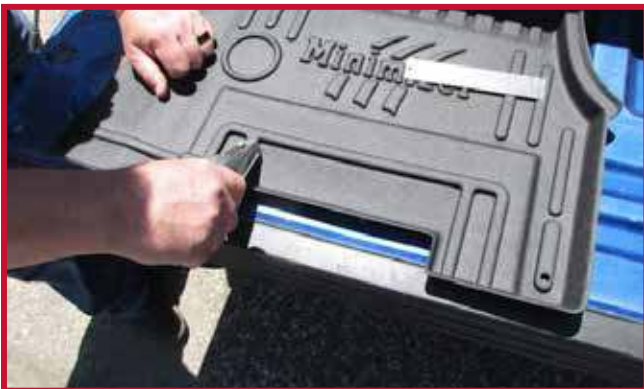
Figure 5 - Hand Trimming the Driver Mat for a Custom Seat Position
