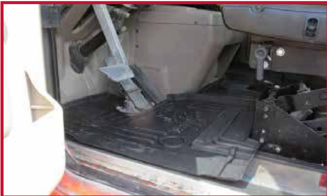
Figure 5 - Hand Trimming the Driver Mat for a Custom Seat Position
