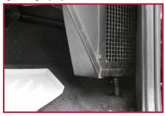
• For Western Star models 4900SA, 4900FA, 4900SB, 4900SF years 1998 - 2011 the yellow shaded area shown in Figure 12 will likely need to be hand trimmed along the raised rib at the time of installation. Test fit the mat before trimming to confirm.
