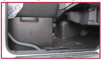
Figure 14 - Fixed Base Passenger Seat with Trimmed Mat
