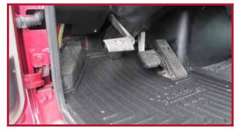
• The driver mat is designed to fit the most common OEM seats. Trucks that are equipped with non-standard aftermarket seats may require hand trimming at the time of installation. If needed there is a raised rib molded into the driver mat to use as a trim guide. The area shaded blue shown in Figure 7 is the portion to be removed. Use a sharp utility knife to remove this portion.
