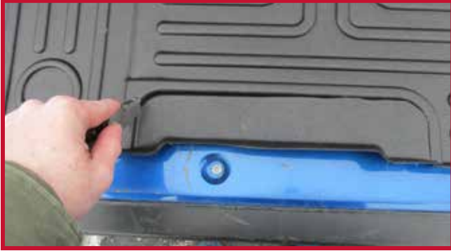
Figure 7 - Driver Mat Trimming Diagram
