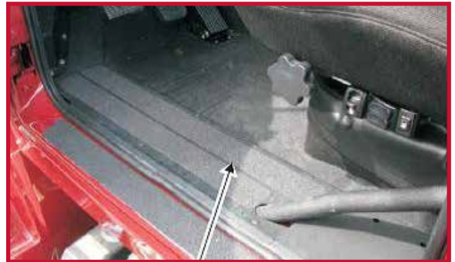
Figure 4 - Driver Side Electrical Tray
