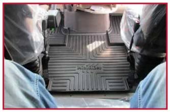
Note: the passenger side floor mat is designed to accommodate both fixed seats and suspension seats. For trucks equipped with a fixed passenger seat, there will be a gap of approximately 1.5 inches between the base of the seat and the back edge of the passenger floor mat.
