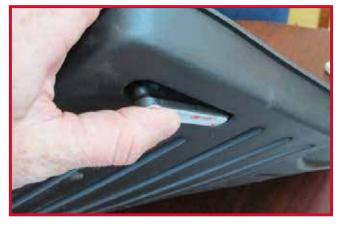
8. Once the hook is in place, let the mat and hook rest on the floor as shown in Figure 6. Next, confirm that the mat is not interfering with foot pedals and verify it is making proper contact with the surfaces surrounding the floor.
