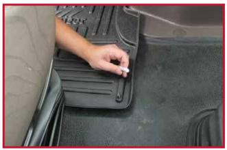
9. Mark the approximate position where the hook will need to be attached to the floor with a finger. Once the position is located, remove the driver mat from the truck.
