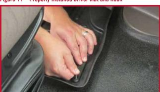
15. Position the passenger floor mat in the truck. Make sure the passenger mat is pushed all the way forward so the outside lip makes full contact with the doghouse trim panels.
