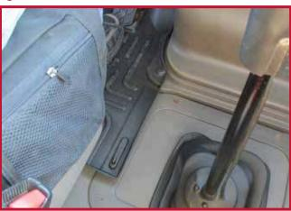
Mark the approximate position where the hook needs to be attached to the floor. Once the position is located, remove the driver mat from the truck.
