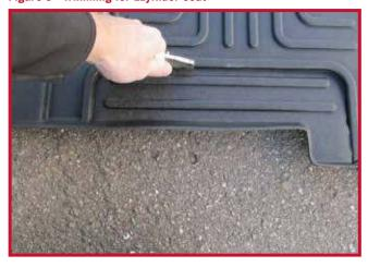
CAUTION: Minimizer floor mats are designed to be used with the factory rubber flooring in good condition. If the factory floor is in poor condition (has humps or bubbles) due to excessive moisture, the floor mat may not sit in place properly. If the floor mat does not sit in place properly there is risk that the floor mat will interfere with the brake and throttle pedals.
