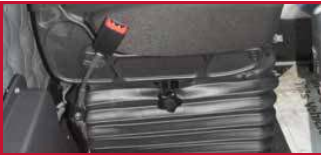
Figure 11 - Hand Trimming for Seat with Rubber Boot
