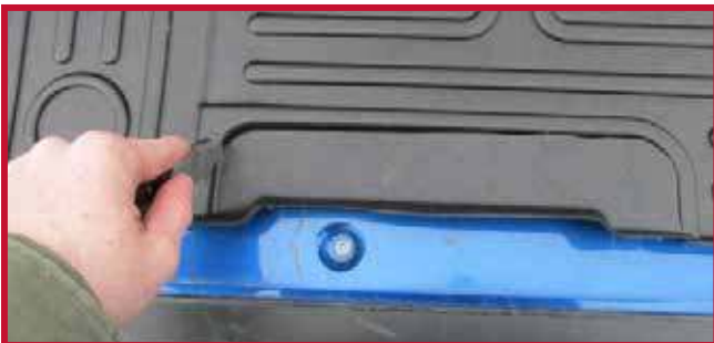
Figure 11 - Hand Trimming for Seat with Rubber Boot
