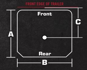
$\mathsf{KP}$  Setback = Measurement from the front edge of the trailer to the center of the king pin.
