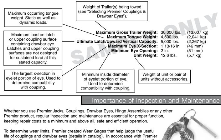
and the Federal Motor Carrier Safety Regulations, these were designed to identify wear at the critical percentages of 18% and 20%, by measuring the crosssection of coupling hooks (horn) and drawbar eye loops. 18% wear indicates that the product should be replaced as soon as possible. At 20% wear, the product is no longer
